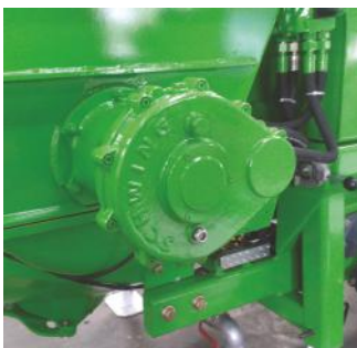
Gearbox drive for agitator
